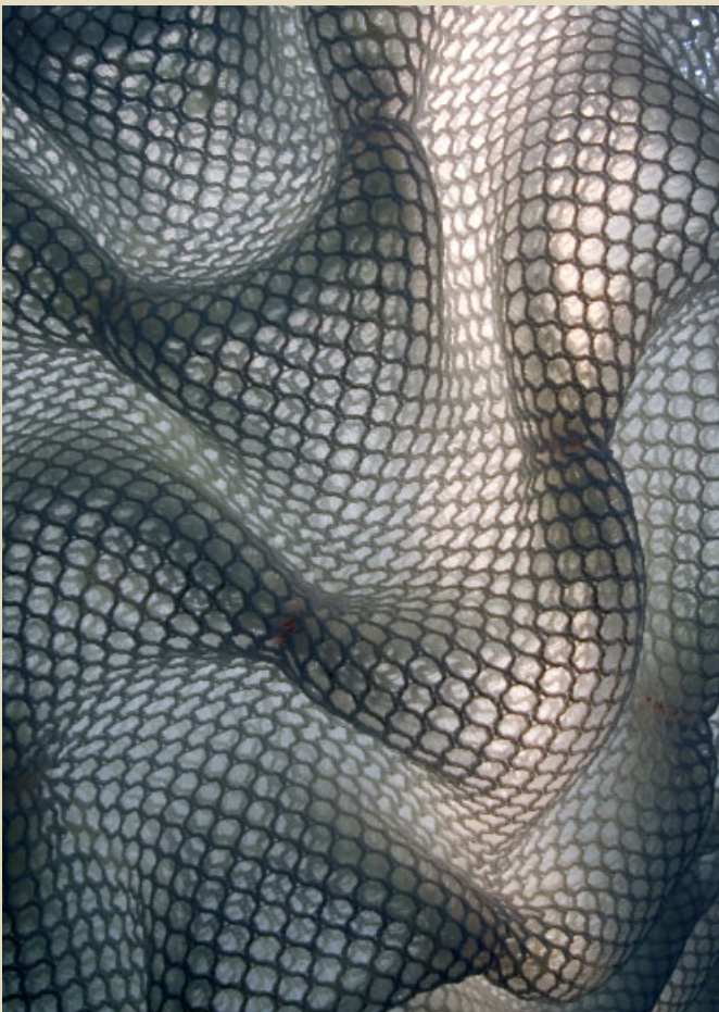
The parametric definition of gathering techniques of a 3-D spacer textile allows for the differential manipulation of primary surface geometry in relation to secondary surface articulation.
