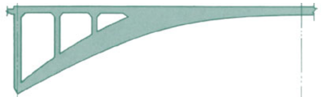
Robert Maillart, Salginatobel Bridge, near Schiers, Switzerland, 1930 The overall geometry of the arch was developed using graphic statics in response to the self-weight of the bridge. The thickness of the arch increases towards the quarter span and tapers towards the crown and supports to control asymmetrical moments due to vehicle movements.
