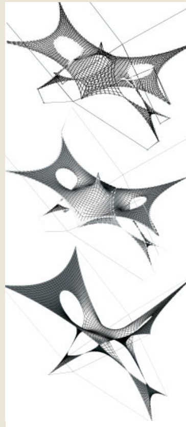
A digital membrane component set up through combined processes of digital dynamic relaxation and parametric modelling. The geometric constraints of the component are derived through the mapping of possible adjustment ranges of the related physical model.
