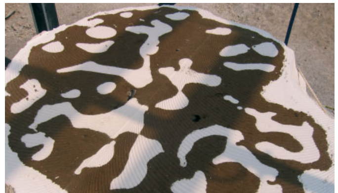
Cross-section from the scanned mound showing how the gypsum infill produces the threshold required for the computer to derive and assemble the final 3-D model.
