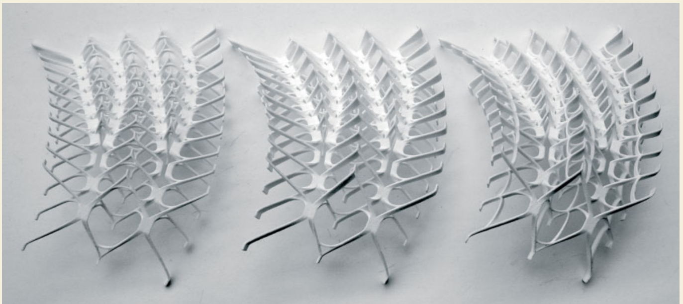
Three different rapid prototype models produced through selective laser-sintering (top) show the geometric adaptation of a multi-component system in response to particular parametric settings (centre) and the resulting performative capacity of the system interacting with a simulated luminous environment (bottom).
