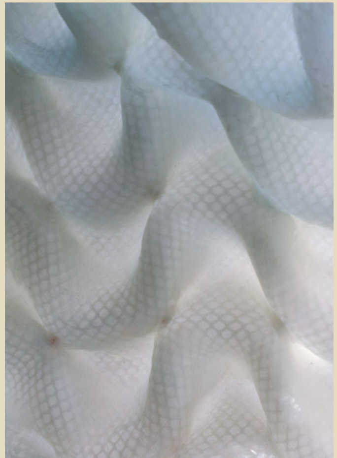
A close-up view of a full-scale prototype shows how local spacer-textile manipulations can be embedded in a glass-fibre composite. The resulting surface integrates both the load-bearing capacity of the structure and the environmental modulation of the skin.
